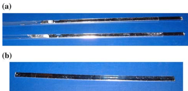
Fig. 7 Solder uniaxial test specimens. a Within glass tubes, b after extraction
